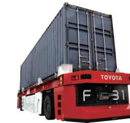
TOYOTA Container Transport AGV System
