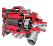
Air Compressor used in the Mirai
