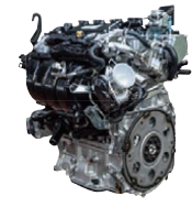
A25A-FKS Displacement: 2.5 liters used in the RAV4
